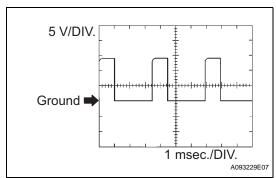
\*1: The ECM terminal voltage is constant regardless of the output voltage from the sensor.
